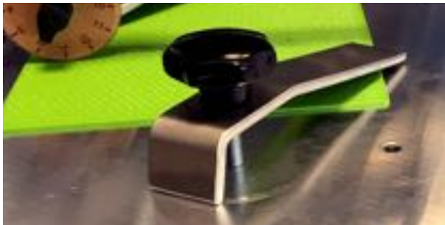
Universal Sample Clamp for flat and curved samples with various height
